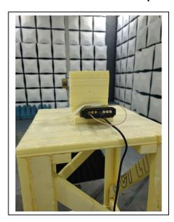
Radiated Emissions Test Setup: Antenna
