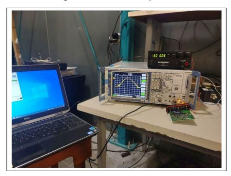
**Voltage Variations Test Setup: Low Voltage (4.7VDC)**
