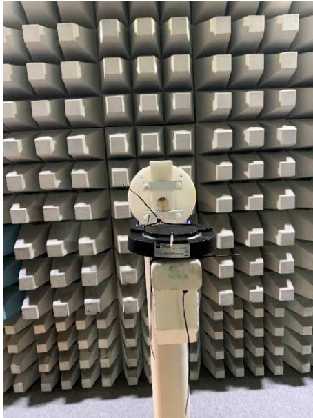
0° Position to measuring antenna
