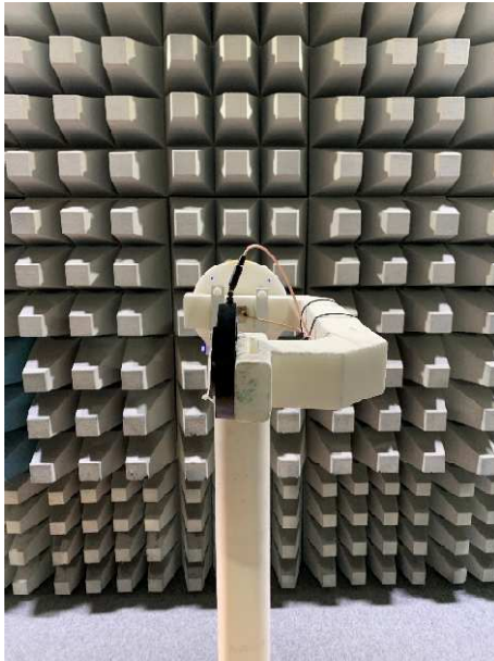
0° Position to measuring antenna
