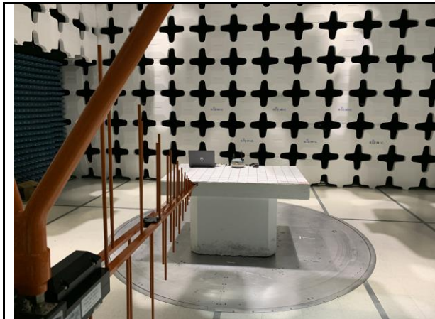
Radiated Emission Test below 1GHz Front View
