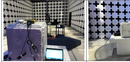
Radiated Emissions above 1GHz – Front View
