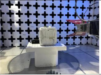
Radiated Emissions above 1GHz – Rear View
