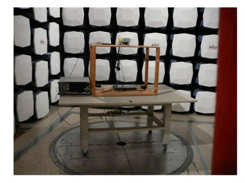
14.1 Radiated Emissions below 1 GHz (Host Orientation: Flat on Table) - Front View
