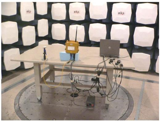
7.2 Transmitter Radiated Emissions – Rear View (Antenna Model: Mobile Antenna)
