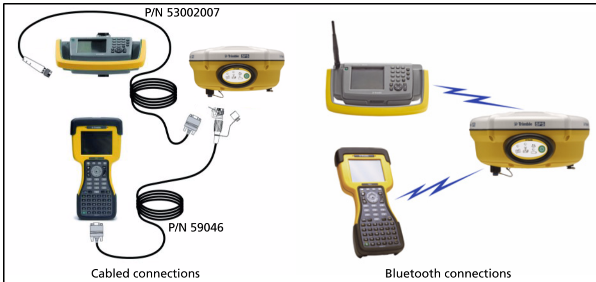
Figure 5.6 Connections for a rover SPSx81 setup, a TSC2 or TCU controller, and a 450 MHz base station
