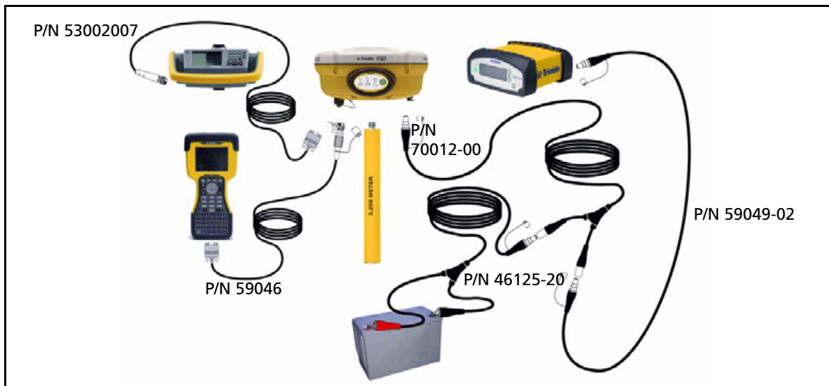
Figure 5.7 Cabled connections for an SPSx81 setup, a TSC2 or TCU controller, and a 900 MHz base station (with external power)
