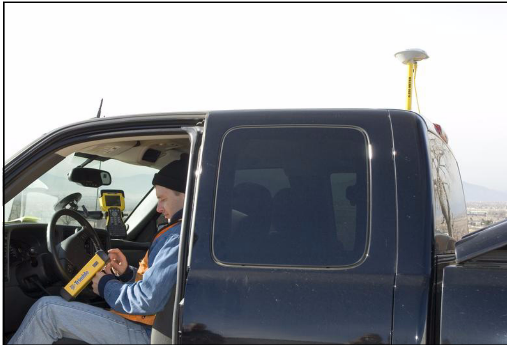
Figure 5.5 Configuring an SPSx50 from the cab. A Zephyr Model 2 antenna is mounted on the roof.
