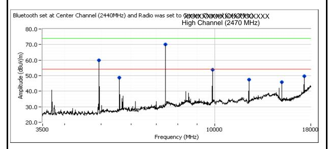
Fundamental Signal Field Strength: Peak and average values measured in 1 MHz, and peak value measured in 100kHz
