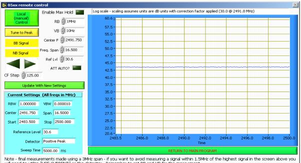
Note - final measurements made using a 3MHz span - if you want to avoid measuring a signal within 1.5MHz of the highest signal in the screen above you will need to utilize "USE CURRENT" as the detector. Remember to set RB and VB for the measurement.
