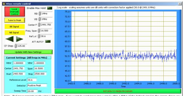
Note - final measurements made using a 3MHz span - if you want to avoid measuring a signal within 1.5MHz of the highest signal in the screen above you will need to utilize "USE CURRENT" as the detector. Remember to set RB and VB for the measurement.
