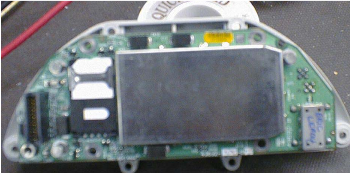
EUT – Internal view showing shielded GSM module
