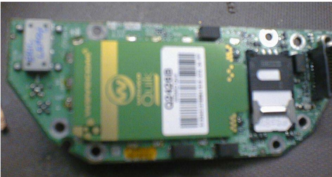
EUT – Internal view showing unshielded GSM module
