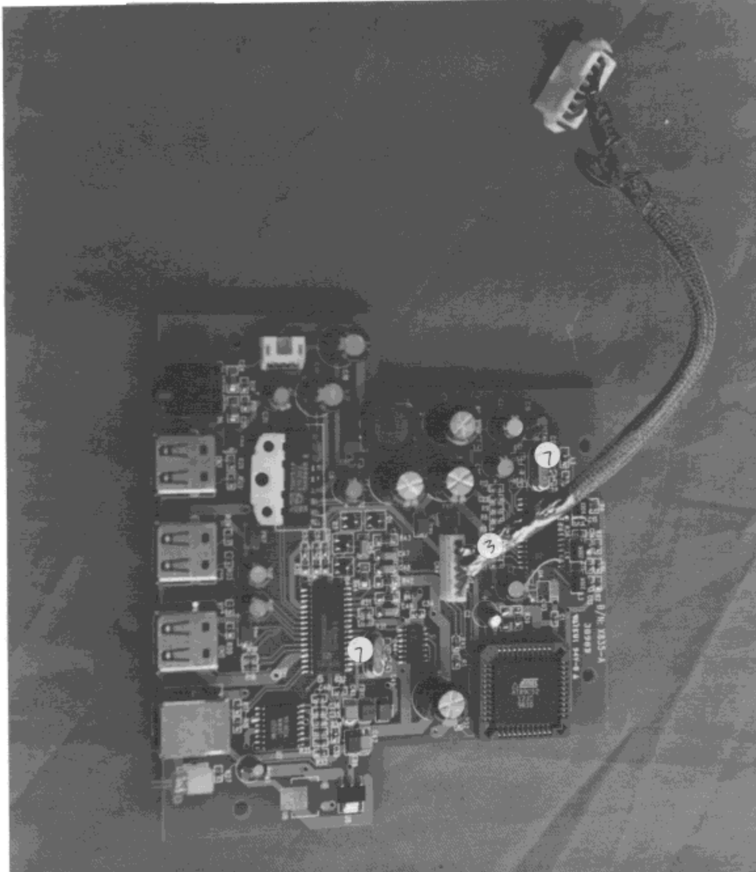
Figure 14 Component Side, USB-Audio PCB
