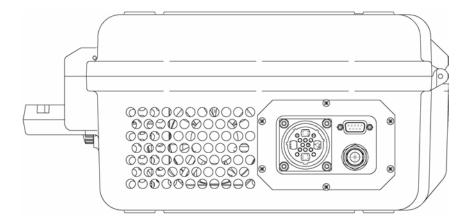
The **Power Connector** (AC or DC Power Cable) and the **RF Connector** (Type N Female) are located on the side panel. The DB-9 connector is used by Grayson Wireless for internal test purposes and has no user function.
