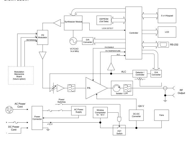
The RF signal is generated in the synthesizer module, which derives its reference from an on board TCXO. The synthesizer tunes in steps appropriate for the frequency band. Following the synthesizer is an I/Q modulator, included for future applications requiring modulation.
