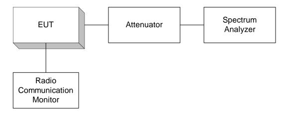
The Radio Communication Monitor is used only to provide modulation input for external modulation.
