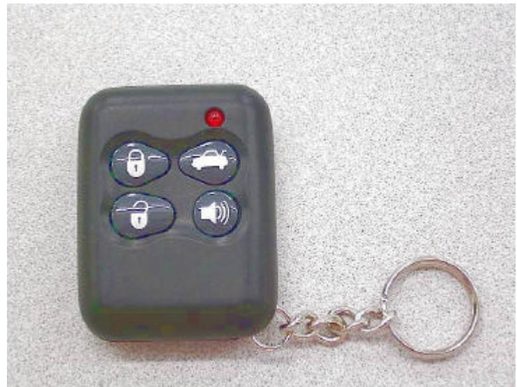
This remote control transmitter provides 2 billions of digital codes with an operative range up to 100 feet, (The operative range will be shorten when system is interrupted or out of power) and also contains Anti-Duplicating & Anti Scanning which is the most secure tool.
