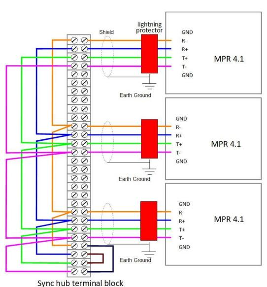
Figure 5-10: Synchronization circuit schematic for three Readers
