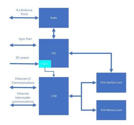
The internal block Diagram is shown in Figure 4-1: MPR 4.1 Block Diagram. The controller Module (CTM) communicates with the Lane Controller and other readers. Through the Channel Group Controller (CGC) the CTM communicates to the radio to interact with Transponders in the capture zone.
