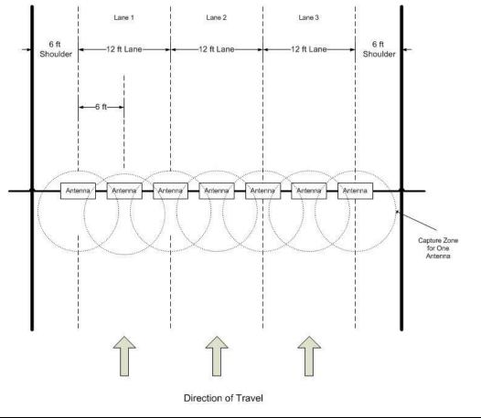
Figure 5-7: Inline ORT Antenna Installation
