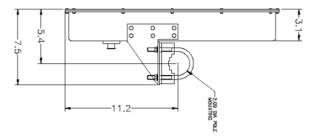
This figure shows the general relationship between the mounting pipe and the antennas. The current antenna drawing should be obtained from Kapsch for accurate dimensions.
