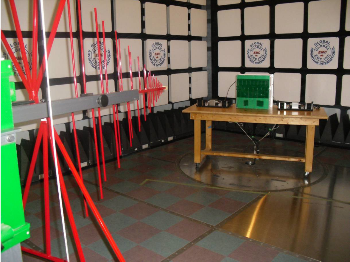
Illustration 6: 802295AA Radiated emission setup – photo 1 Note: 4 instances of 802295AA were present in setup
