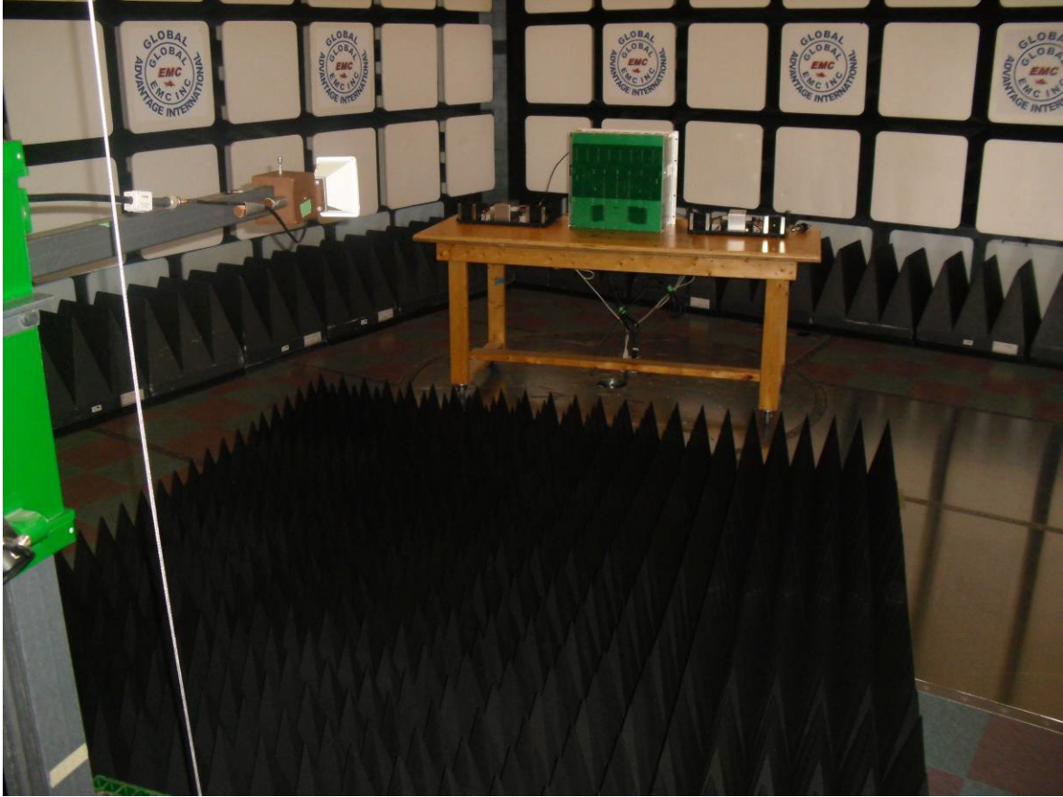
Illustration 7: 802295AA Radiated emission setup - photo 2 Note: 4 instances of 802295AA were present in setup
