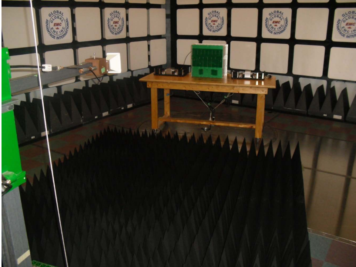
Illustration 2: 802295A-A Radiated emission setup - photo 2 Note: 4 instances of 802295A-A were present in setup
