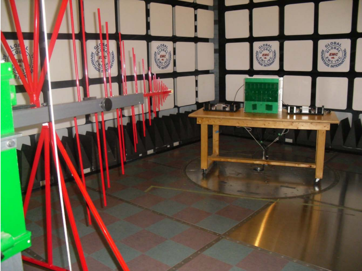
Illustration 1: 802295A-A Radiated emission setup – photo 1 Note: 4 instances of 802295A-A were present in setup
