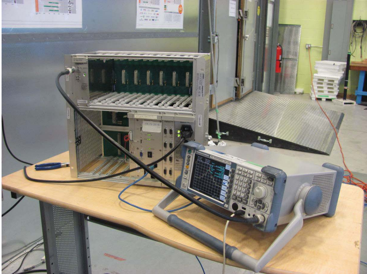
Illustration 4: Antenna conducted emission setup
