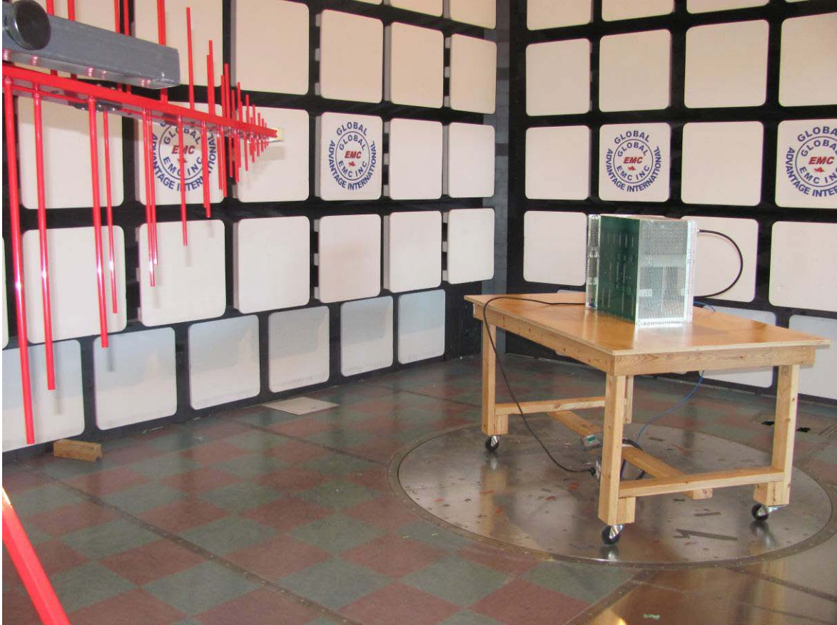
Illustration 1: 802356 Radiated emission setup – photo 1
