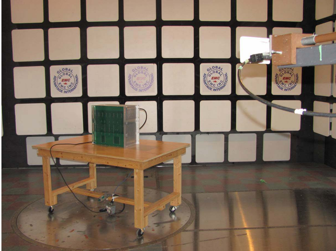
Illustration 2: 802356 Radiated emission setup - photo 2
