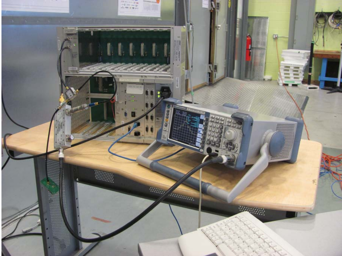
Illustration 5: Antenna conducted emission – KTDM setup with circulator
