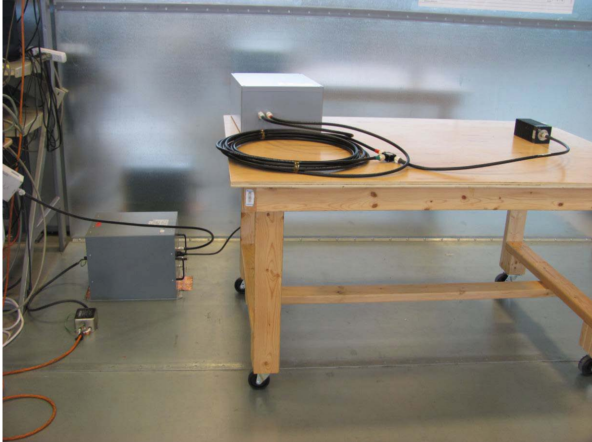
Illustration 10: 802356-TAB Power line conducted emission setup – photo 1
