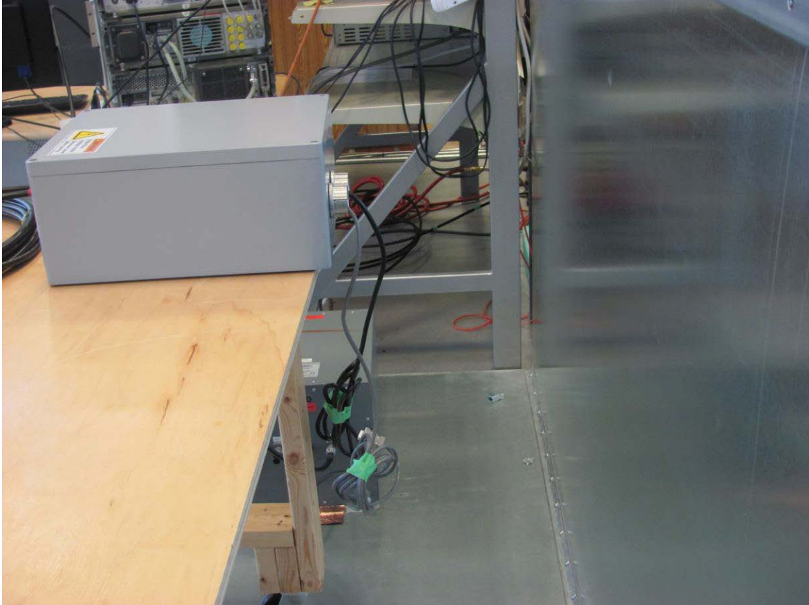
Illustration 11: 802356-TAB Power line conducted emission setup – photo 2
