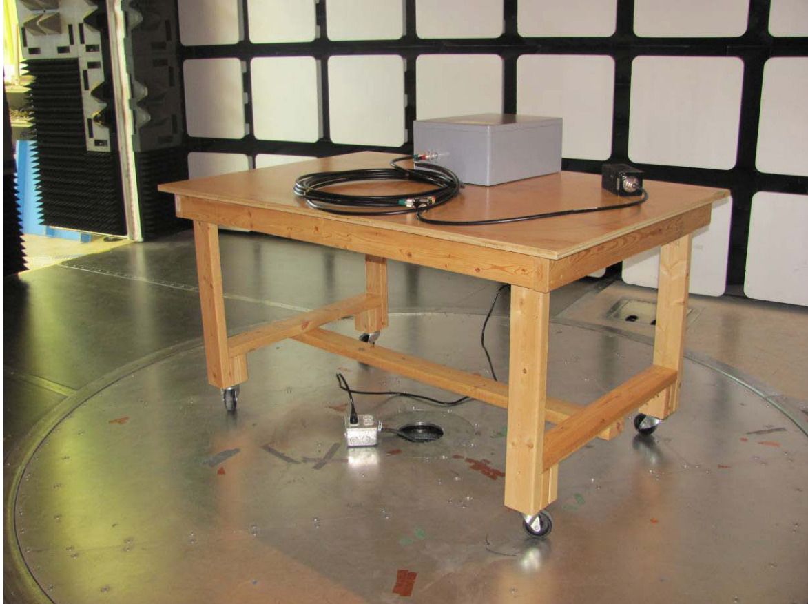
Illustration 7: 802356-TAB Radiated emission setup – photo 1
