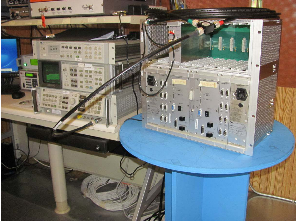
Illustration 4: Antenna conducted emission setup
