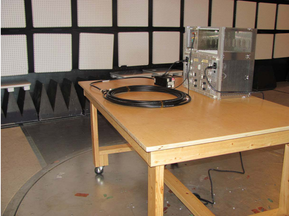
Illustration 1: 802356-TAB Radiated emission setup – photo 1
