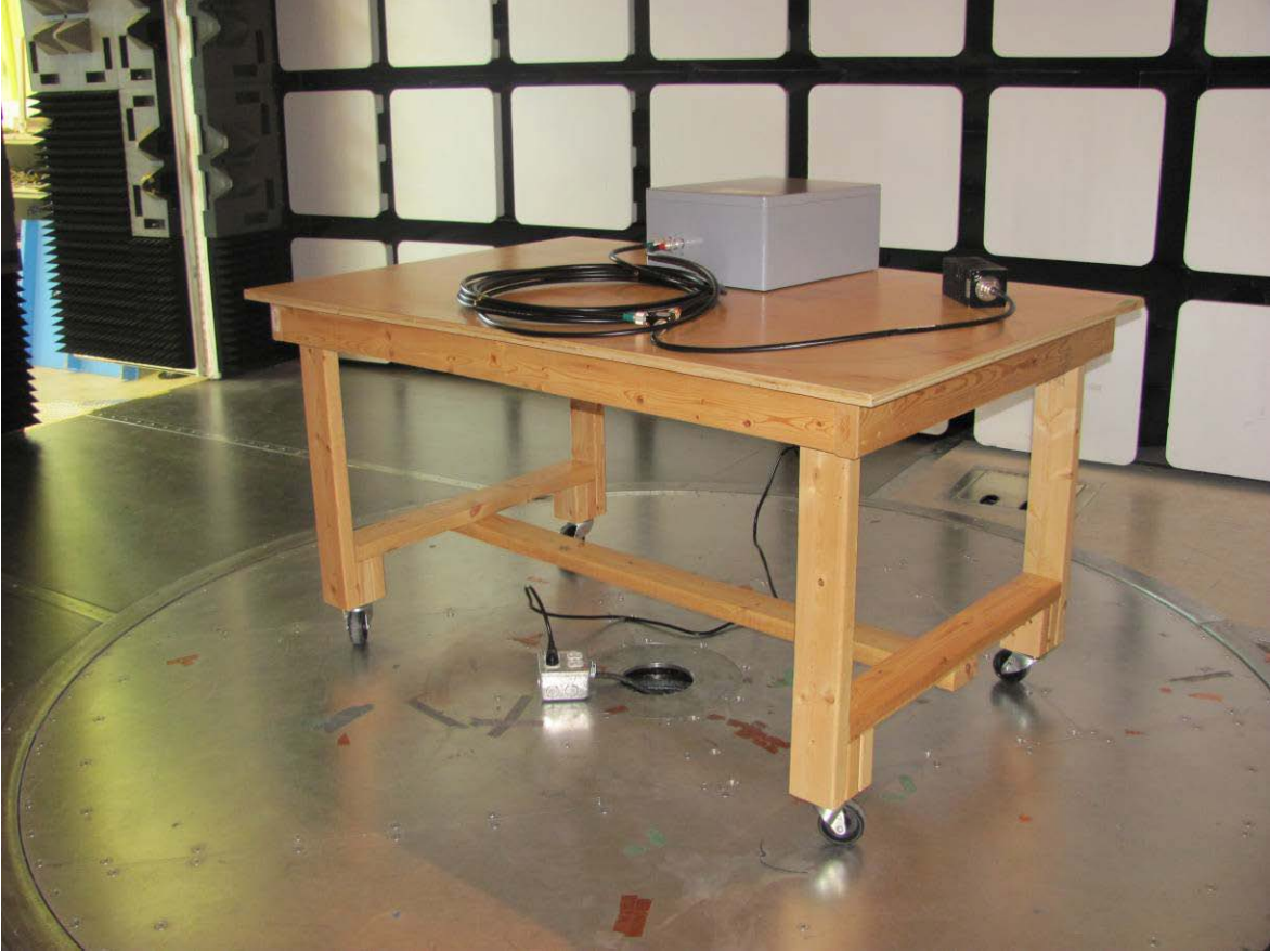
Illustration 11: 802356 Radiated emission setup – photo 1
