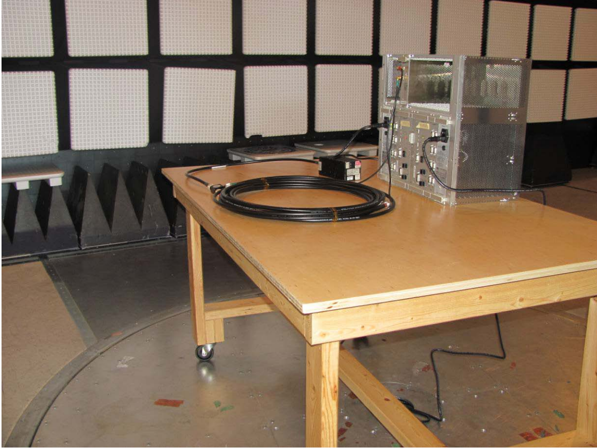
Illustration 5: 802356 Radiated emission setup – photo 1
