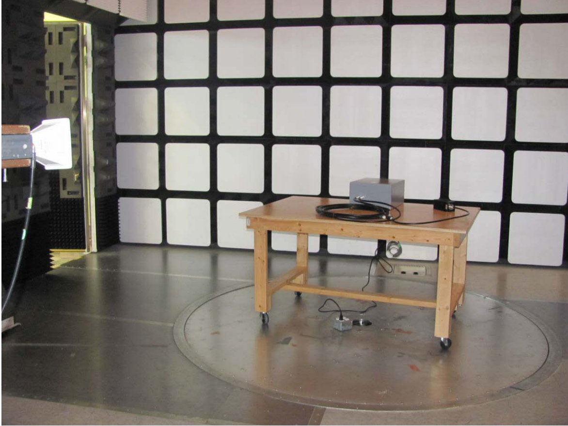
Illustration 13: 802356 Radiated emission setup – photo 3
