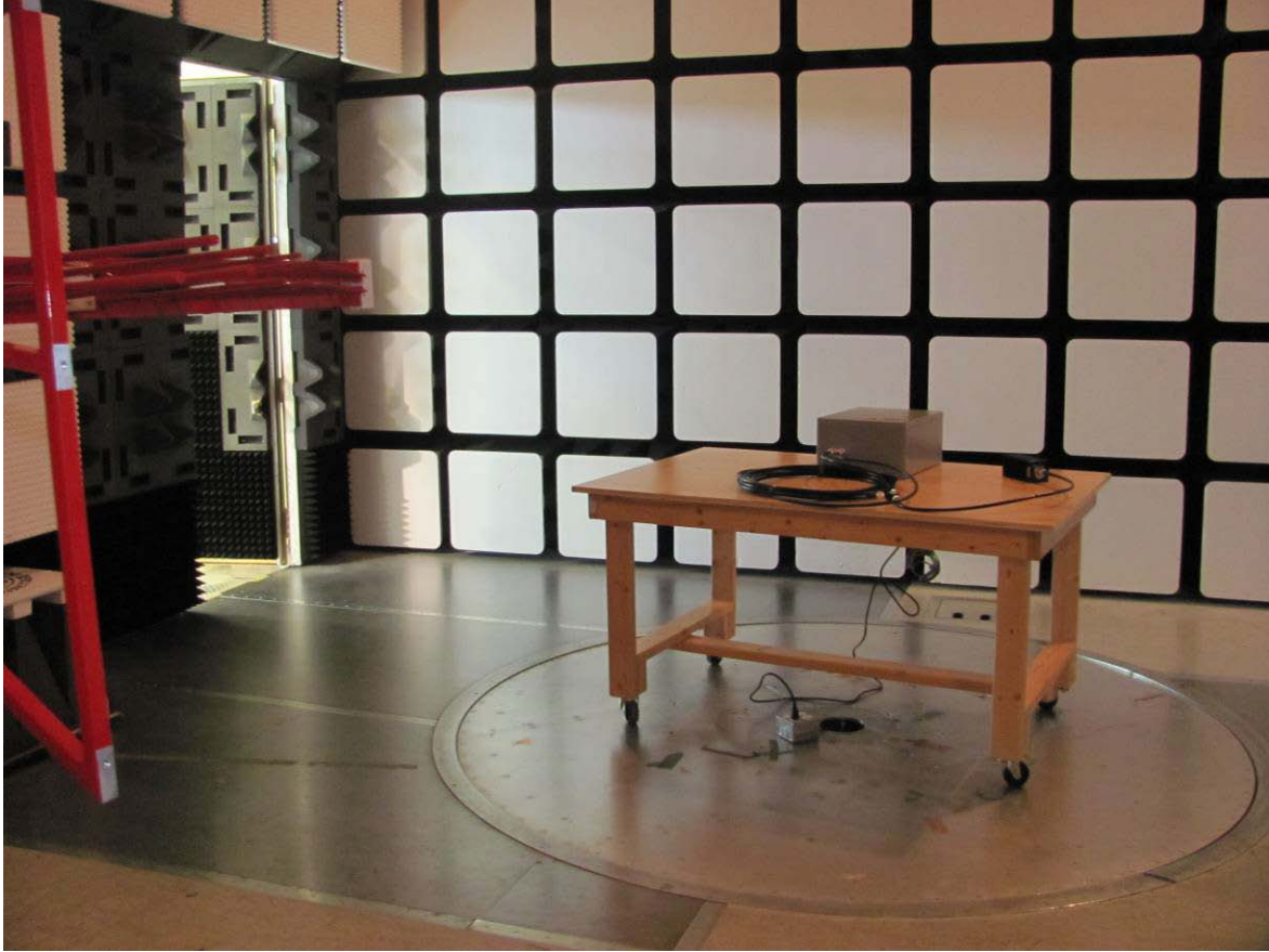
Illustration 12: 802356 Radiated emission setup – photo 2
