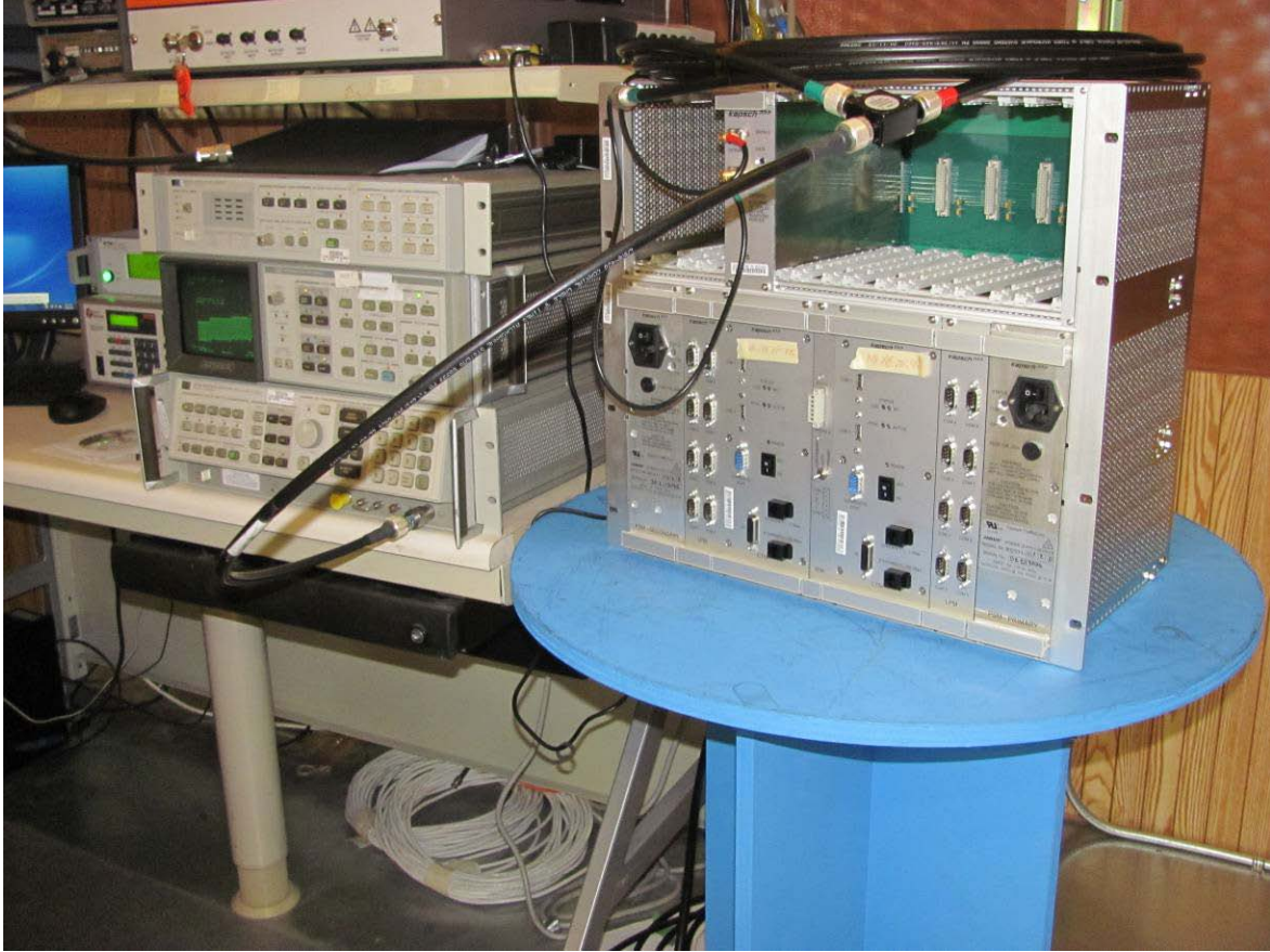
Illustration 8: Antenna conducted emission setup
