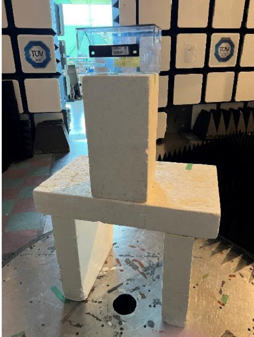
Figure 3 – Radiated Emissions Setup – >1GHz
