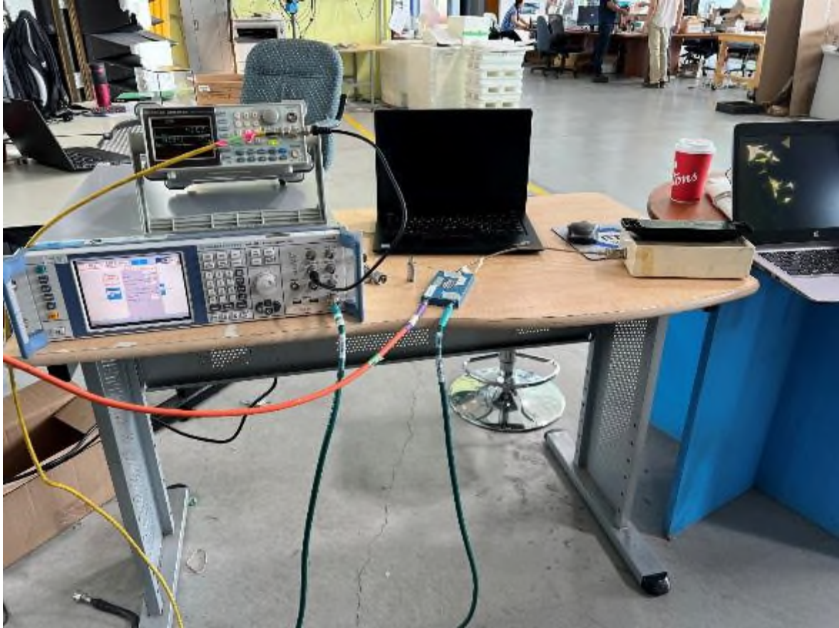
Figure 6 – Antenna Port Conducted Emissions Setup
