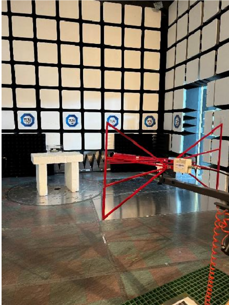
Figure 4 – Radiated Emissions Setup 30MHz – 1GHz
