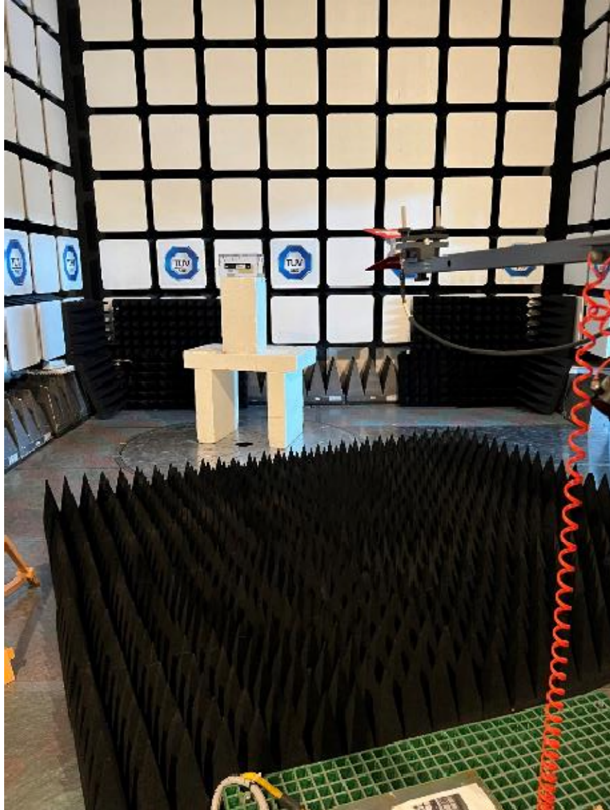
Figure 5 – Radiated Emissions Setup 1GHz – 10GHz
