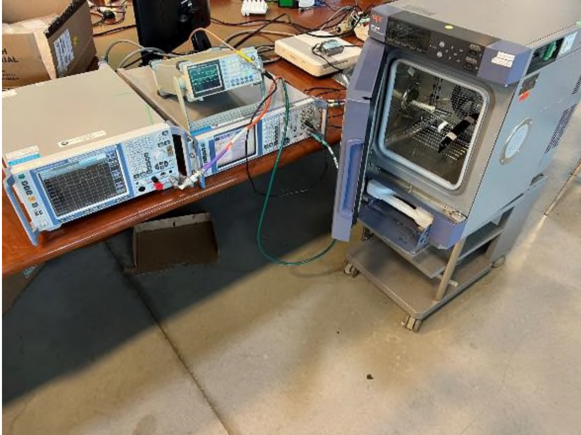
Figure 7 – Frequency Stability Setup
