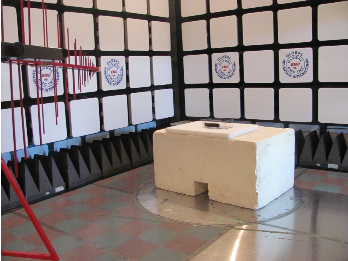
Illustration 3: Radiated emission setup – photo 1
