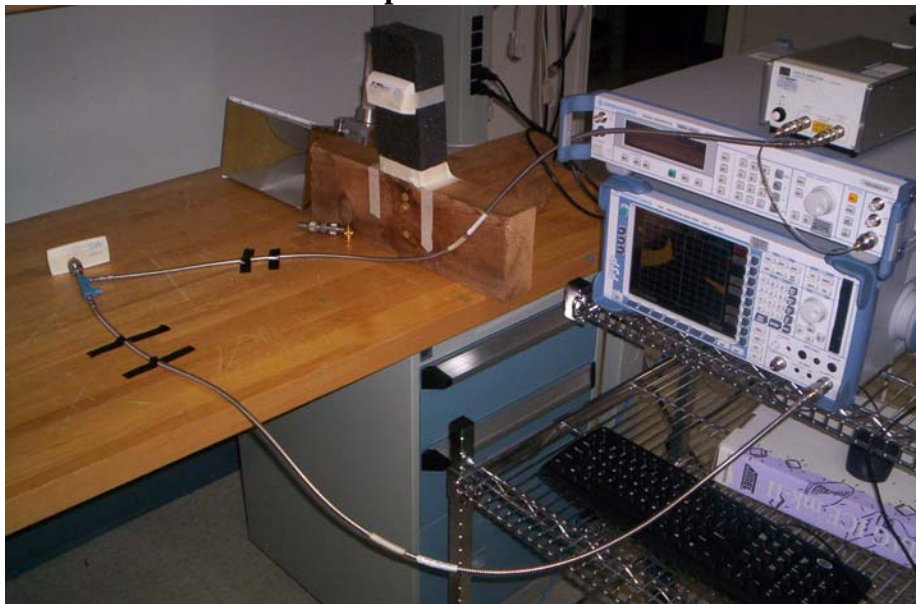
Conducted Emissions Setup:
