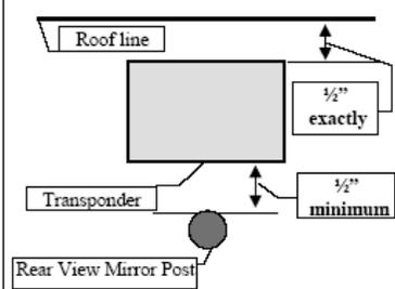
Fig.-3 Alternate Mounting Location
