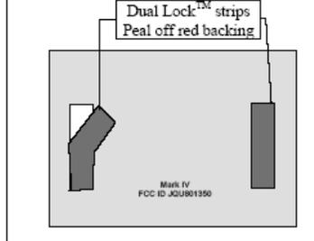
The transponder may be removed by lifting any one corner with sufficient pressure to separate the Dual Lock™ strips. Do not remove the Dual Lock™ from the windshield and reuse it; obtain new strips from your service center if necessary.
