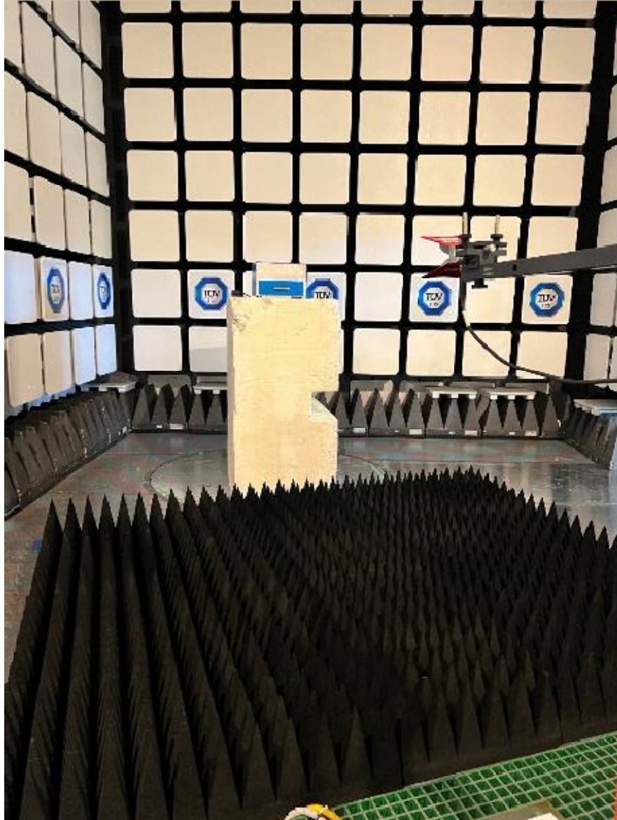
Figure 8 – Radiated Emissions Setup 1GHz – 6GHz
