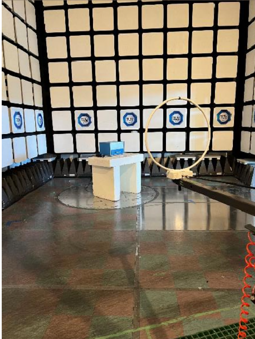
Figure 6 – Radiated Emissions Setup 9kHz – 30MHz
