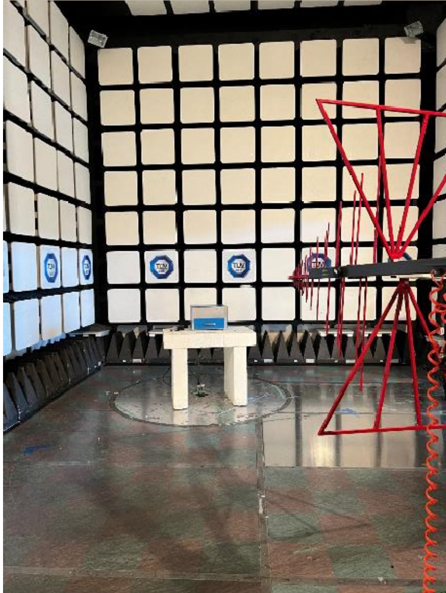
Figure 7 – Radiated Emissions Setup 30MHz – 1GHz
