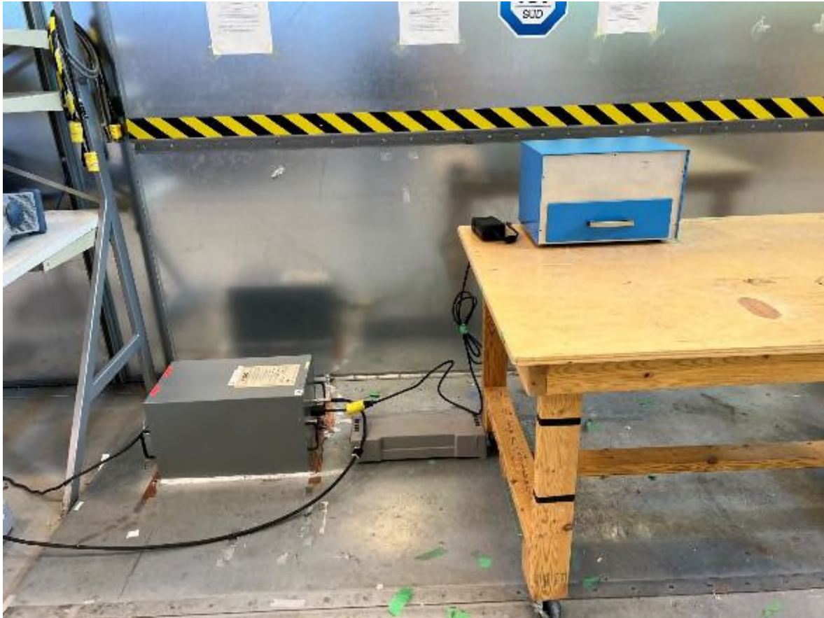
Figure 10 – Conducted Emissions Setup
