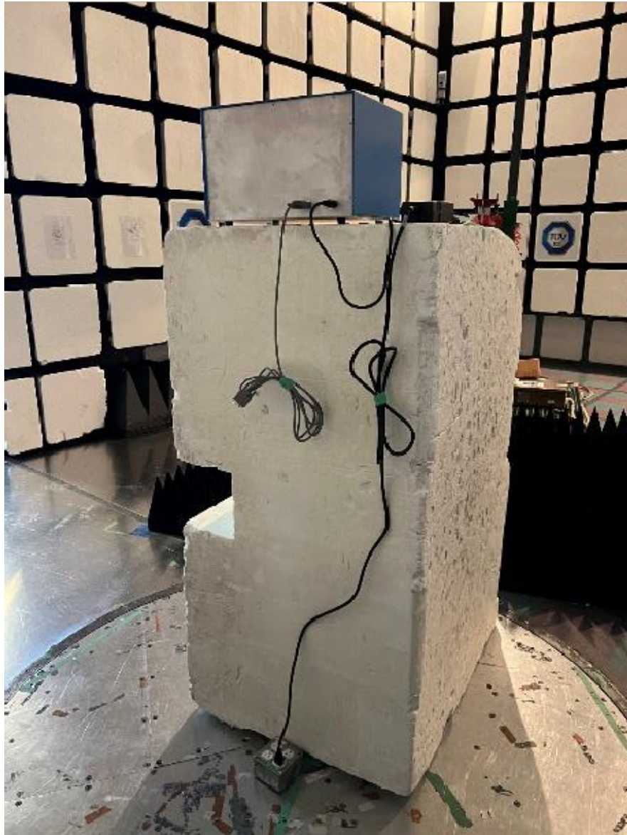
Figure 5 – Radiated Emissions Setup (>1GHz)
