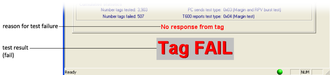
Figure 2-5: Tag Failure Message
