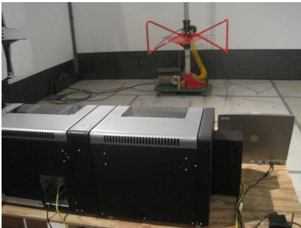
Radiated Emission Test Setup – Rear View
