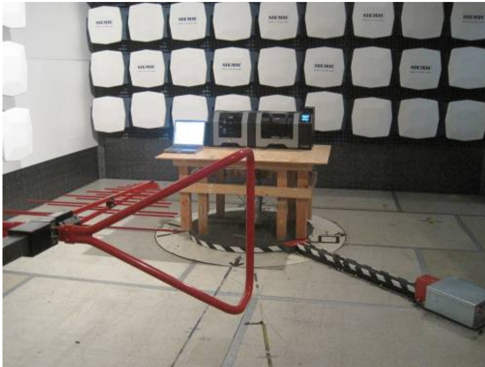
Radiated Emission Test Setup – Front View
