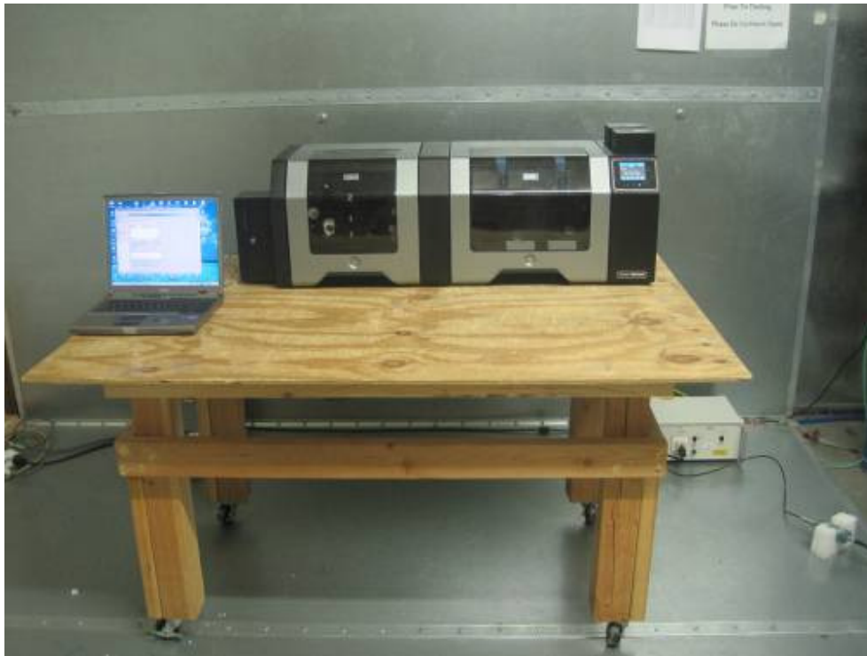
Conducted Emission Test Setup – Front View
