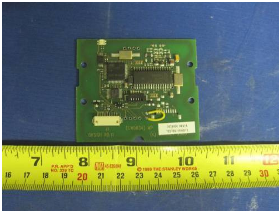
PCB 3 Component View (5121SDI RFID)
