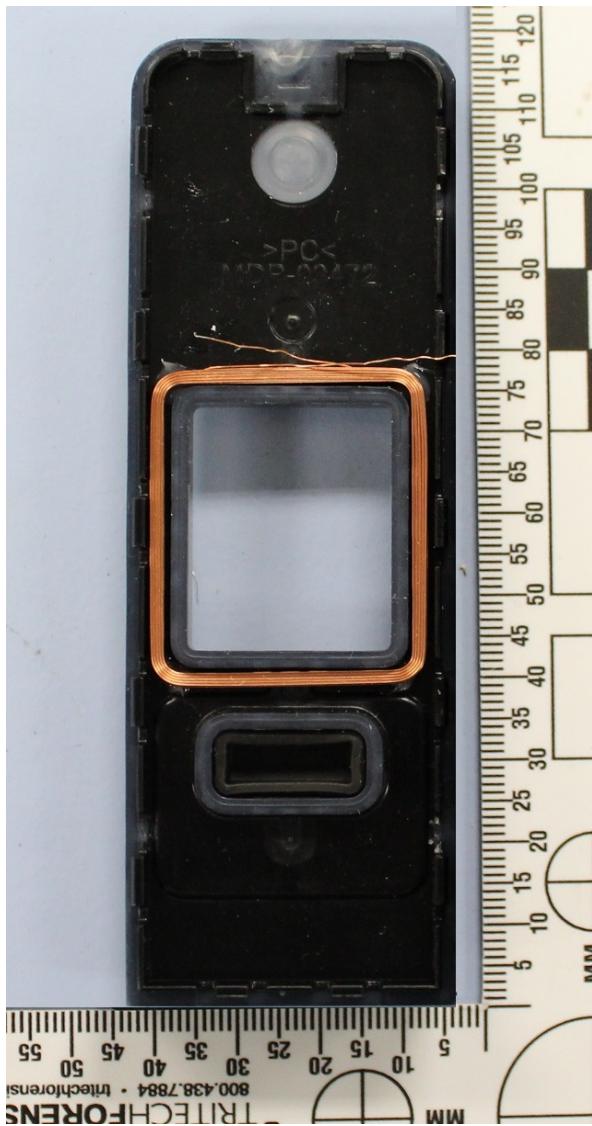
Model 20 (pigtail version) rear cover antenna
