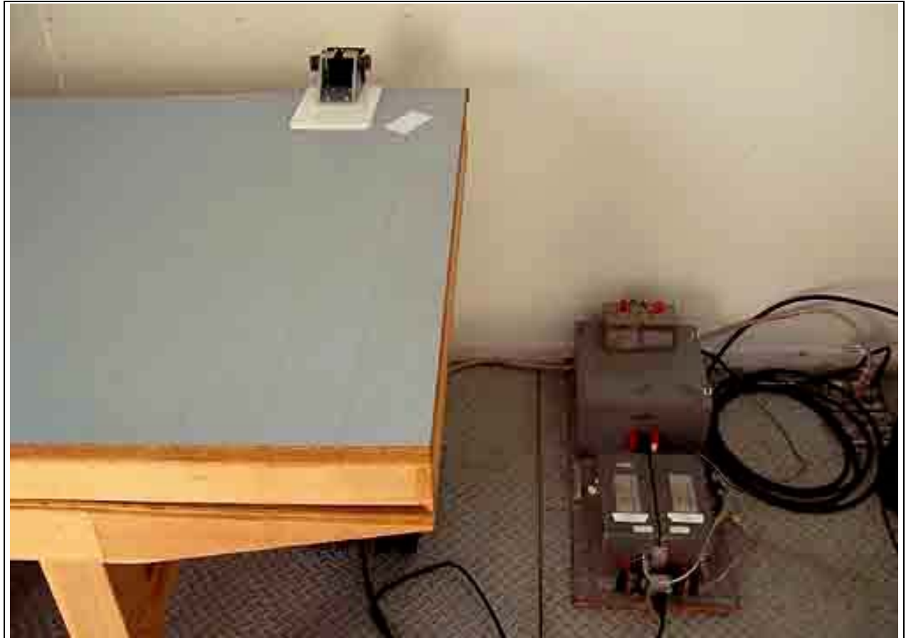
Mains Conducted Emissions - Front View - 6111B
