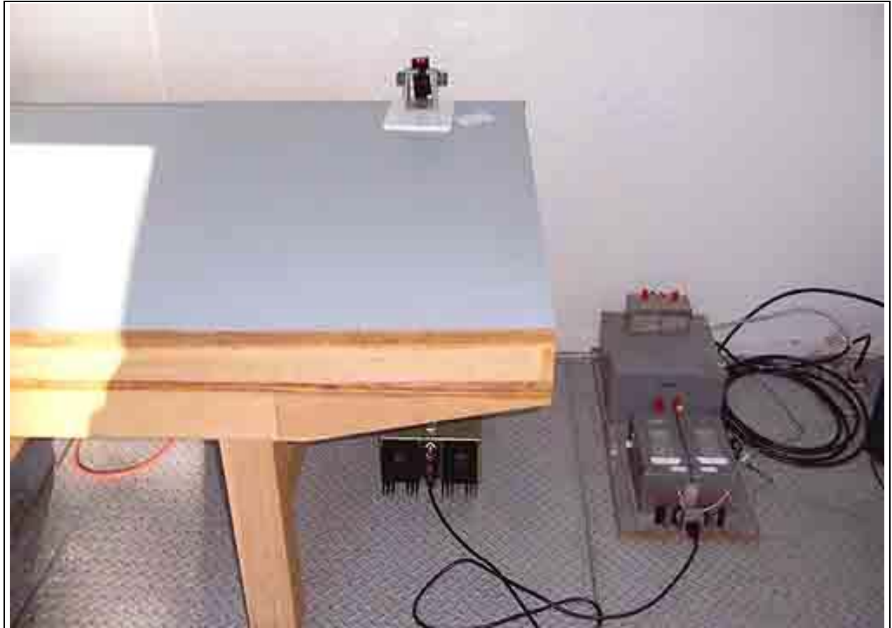
Mains Conducted Emissions - Front View - 6101B
