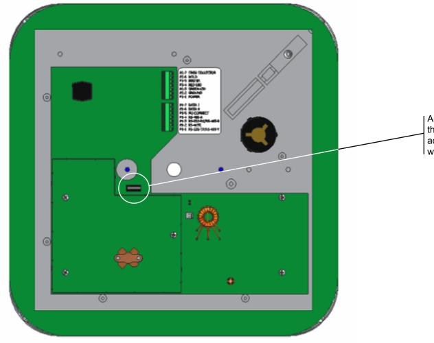
An on board tamper switch is wired through the "I'm Alive" feature and if active, the standard supervisory signal will stop if the cover is removed.
