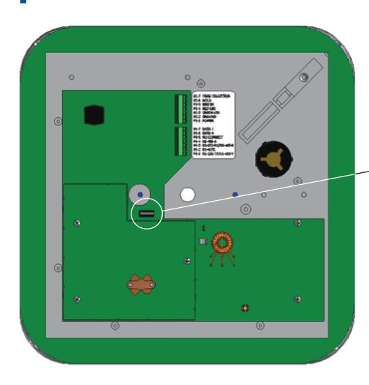
An on board tamper switch is wired through the "I'm Alive" feature and if active, the standard supervisory signal will stop if the cover is removed.
