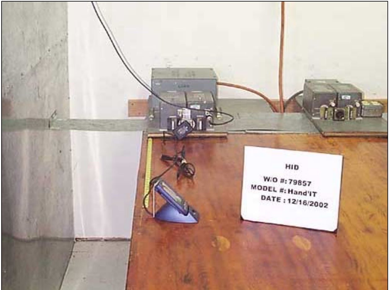
Mains Conducted Emissions - Side View
