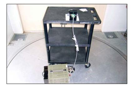
**Test Conditions:** Equipment is a multiCLASS Reader operating on a frequency of 13.56 MHz and 125 kHz. The EUT is mounted vertically on a support structure to simulate normal installation. DC power supply is bonded to ground. 125 kHz transmitter module installed is Prox Module II.
