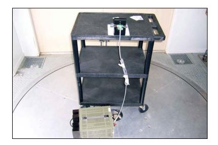
**Test Conditions:** Equipment is a multiCLASS Reader operating on a frequency of 13.56 MHz and 125 kHz. The EUT is mounted vertically on a support structure to simulate normal installation. DC power supply is bonded to ground. 125 kHz transmitter module installed is Indala Module.
