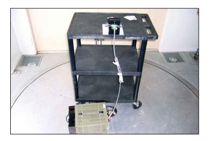
**Test Conditions:** Equipment is a multiCLASS Reader operating on a frequency of 13.56 MHz and 125 kHz. The EUT is mounted vertically on a support structure to simulate normal installation. DC power supply is bonded to ground. 125 kHz transmitter module installed is ASK Module.
