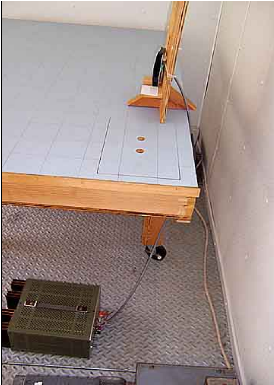
Mains Conducted Emissions - Side View
