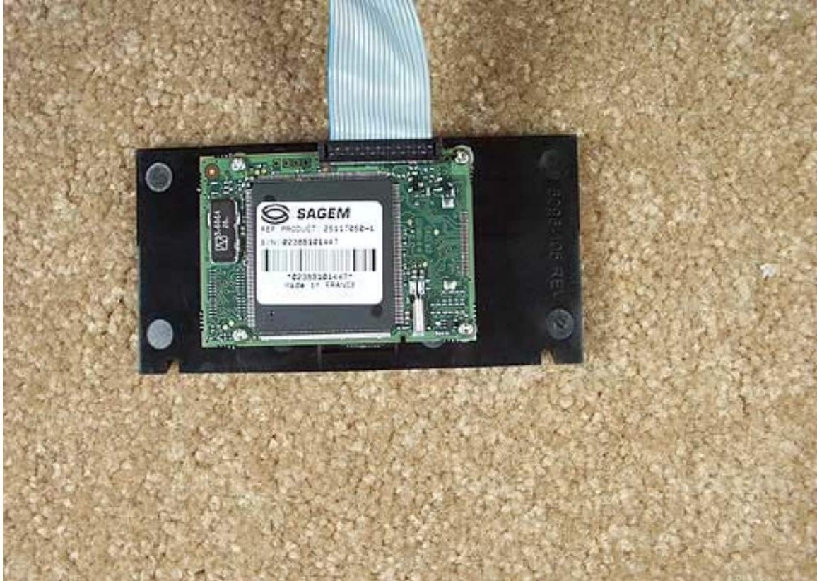
Main Finger Pad PCB Top
