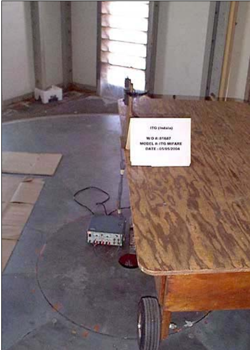
Radiated Emissions - Side View
