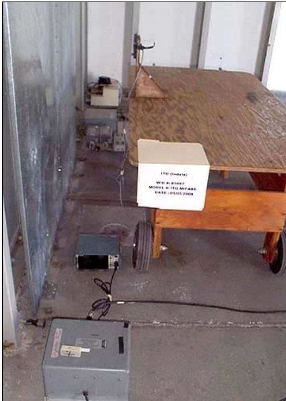
Mains Conducted Emissions - Side View
