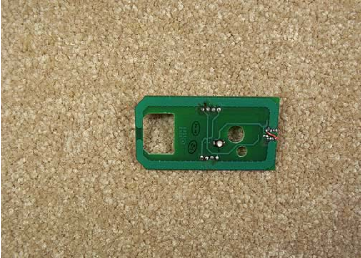
Antenna PCB Bottom
