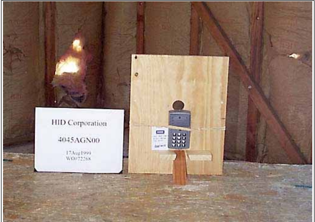
Radiated Emissions - Front View Short Antenna
