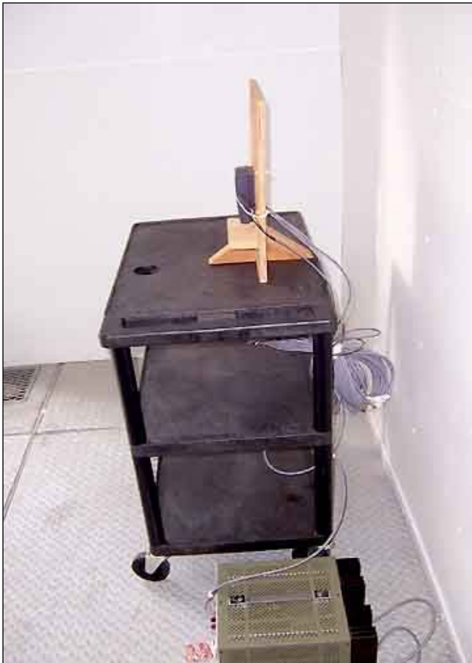
Mains Conducted Emissions - Side View - Remote Antenna
