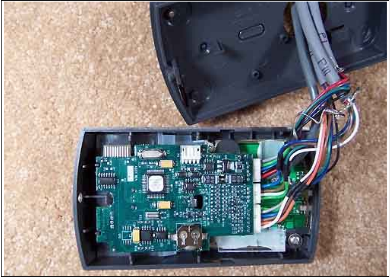
Internal Overall - Remote Antenna
