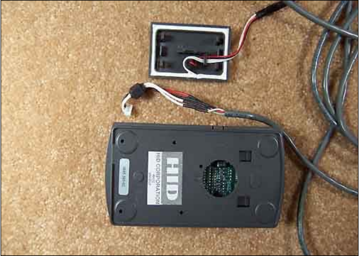
External Back - Remote Antenna
