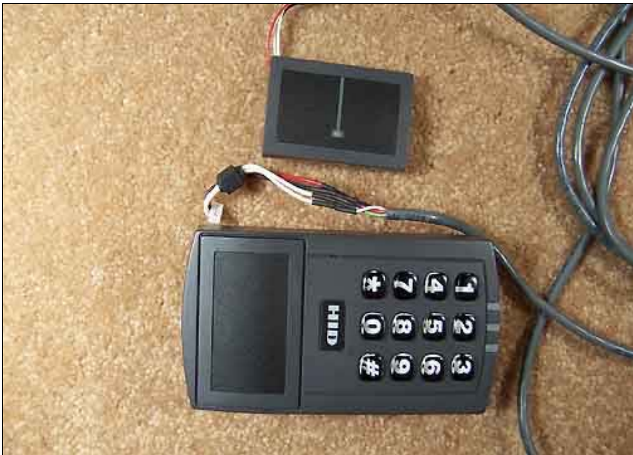
External Front - Remote Antenna
