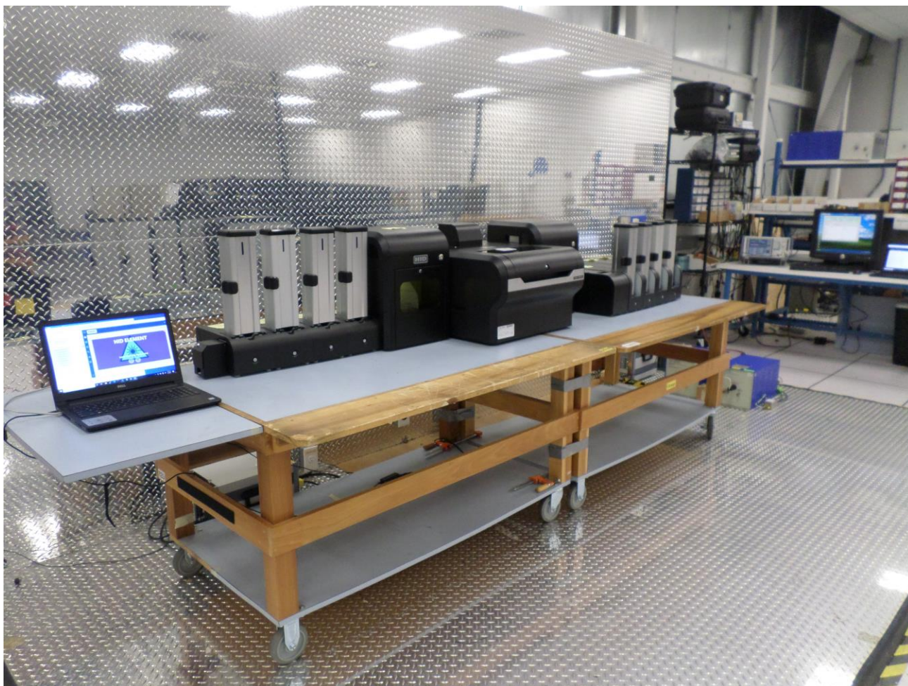
Figure 2: Conducted Emissions, Voltage - Setup Front View
