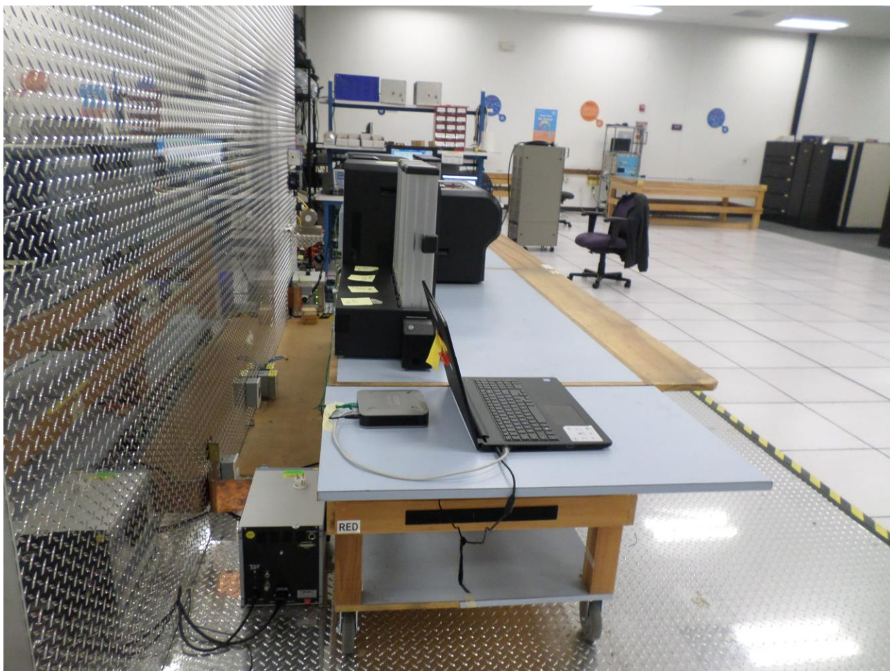
Figure 4: Conducted Emissions, Voltage - Setup Rear View
