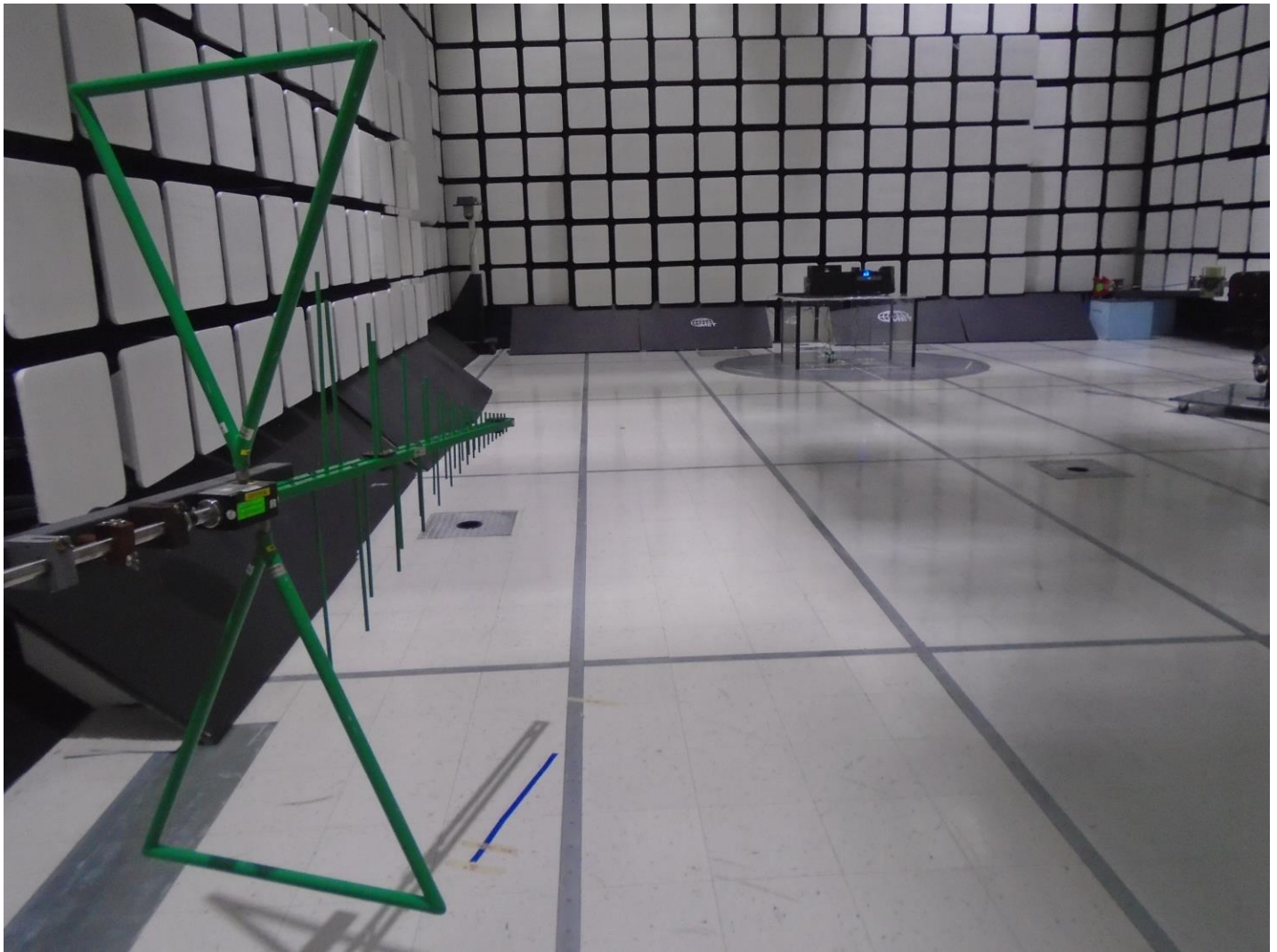
Photograph 1. REE 30-1000 MHz Antenna View
