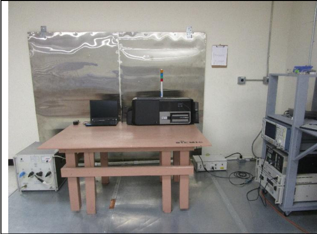
AC Line Conducted Emissions- Front View
