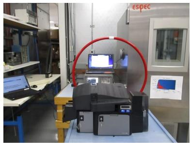
Photograph 10. Emissions Bandwidth Test Setup
