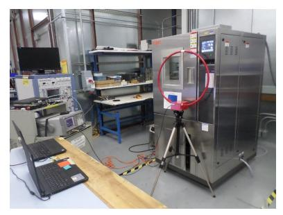
Photograph 9. Frequency Stability Test Setup
