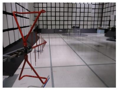
Photograph 8. Field Strength Above 30 MHz, Test Setup Antenna View
