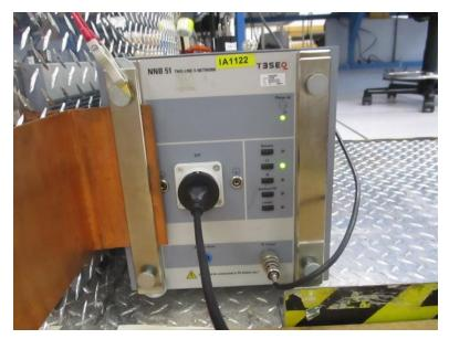
Photograph 3. Conducted Emissions, AC Main, Test Setup LISN View
