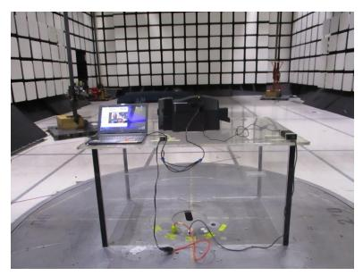
Photograph 7. Field Strength Above 30 MHz, Test Setup Rear View
