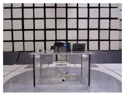
Photograph 6. Field Strength Above 30 MHz, Test Setup Front View
