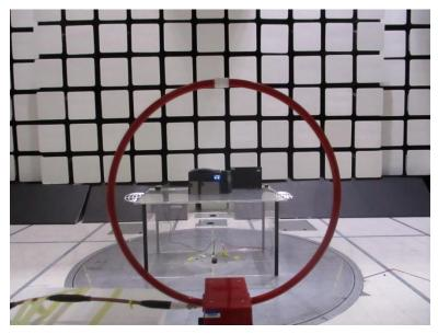
Photograph 4. Field Strength Below 30 MHz, Test Setup Front View
