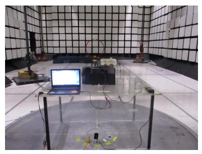
Photograph 5. Field Strength Below 30 MHz, Test Setup Rear View
