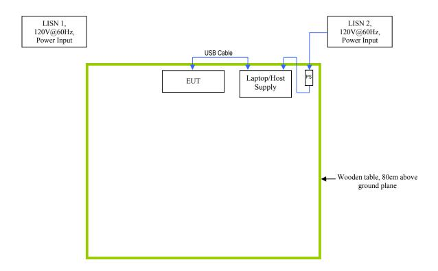
NOTE: EUT was powered by Host using USB as the host interface
