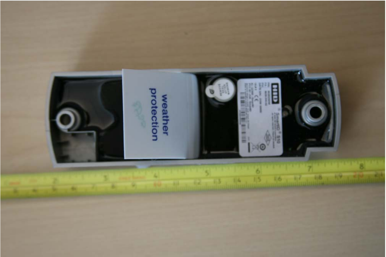
Back showing label placement – Label is placed directly on the potting as shown above.
