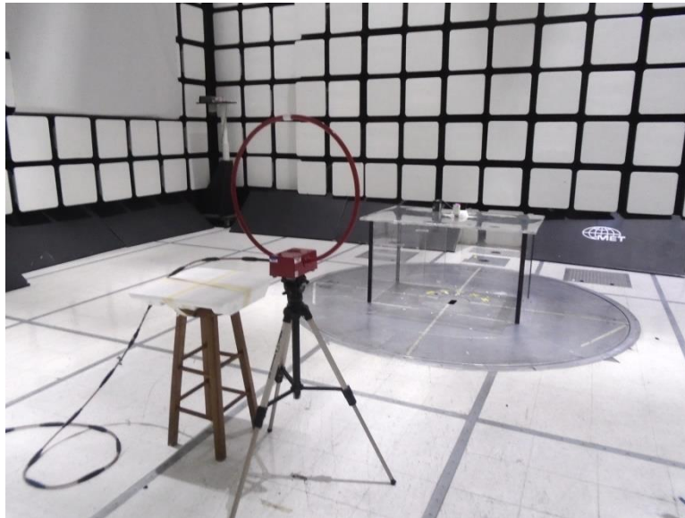
Figure 1: Radiated Spurious Emissions, Test Setup
